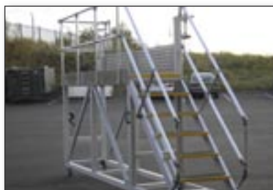
Flask inspection platform
